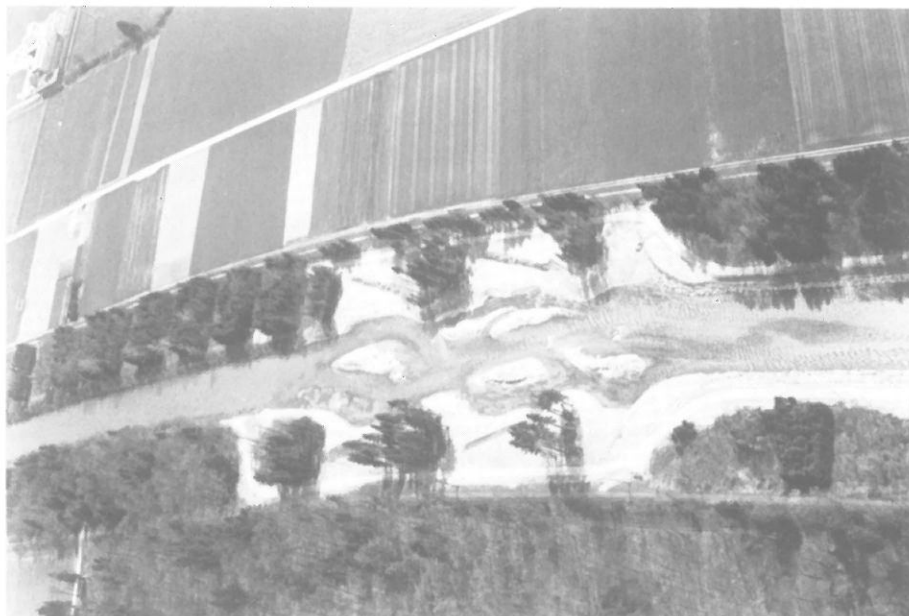
Fig. 9 Local widening in the Emme river (April 1992), an erosion control measure which is at the same time a river restoration
