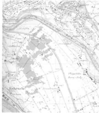
Figure 3-2: Flood layer for 26-May-1999 (dark) obtained from multi-temporal ERS SAR data combined with the geographic map of the area. Grid size is 1 km.
