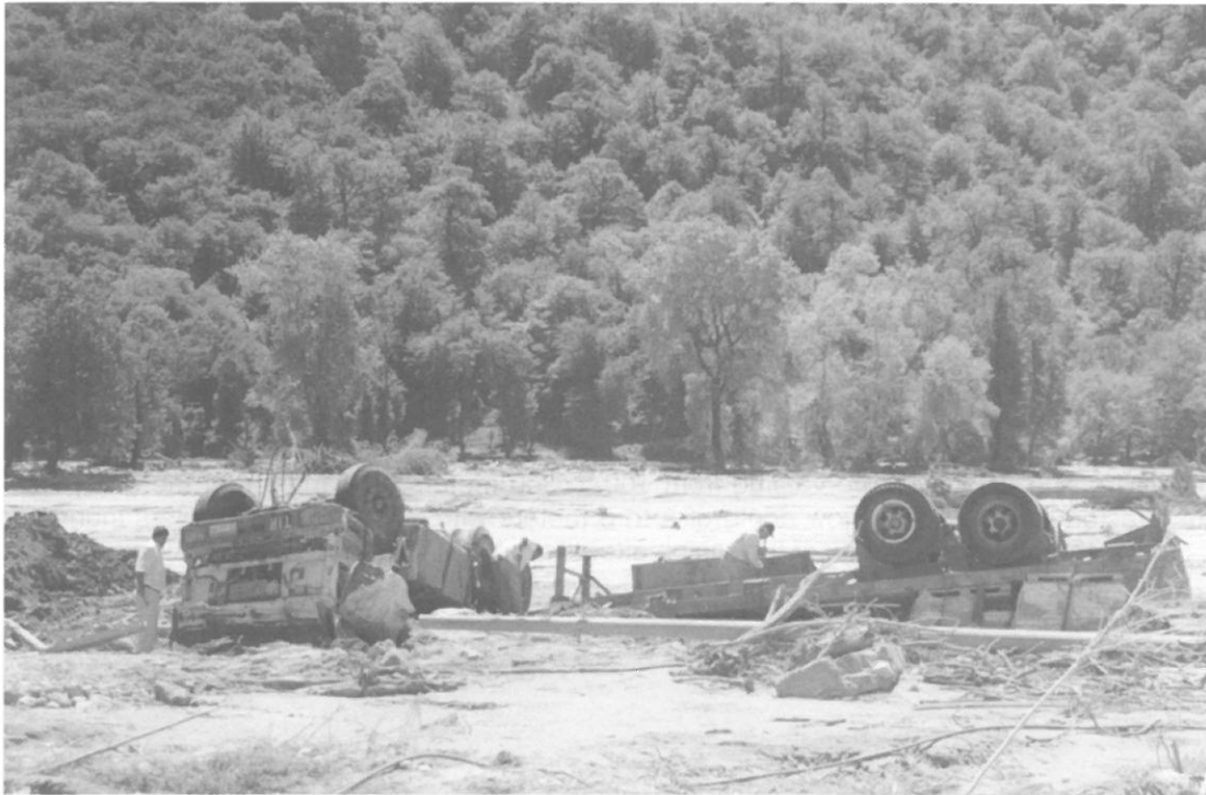
Figure 4-5: Heavy vehicle buried by debris flow.
