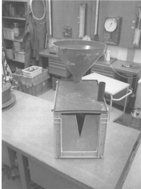
Figure 4-4: Small gauging box that is placed at the bottom of a testplot.
