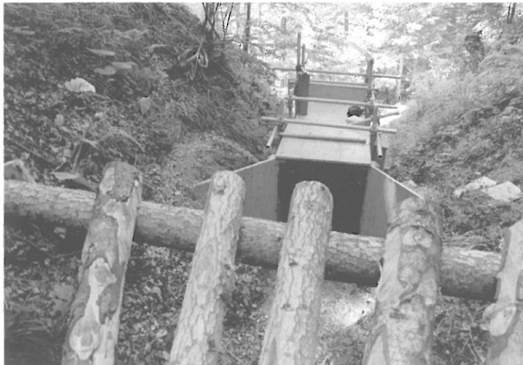
Figure 4-2: View in flow direction on the gauging station of the hardly damaged sub-catchment (grid in the foreground).
