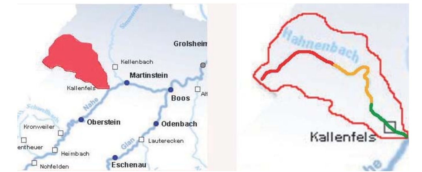
Figure 4 Run-off forecast for a small catchment showing four warning levels (red, orange, yellow, green). The measured water level for a specific point is extended by forecasts in two ways: temporally (e.g. for the next 24 hours) and spatially (i.e. for river sections).
