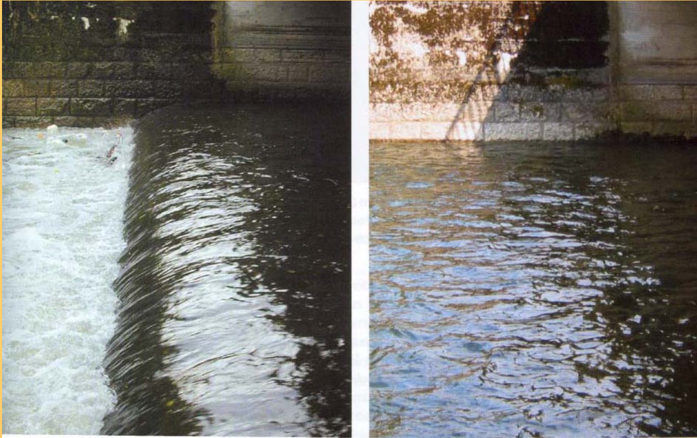
5 m 3 /s in the Glatt River at gage site (left without, right with „Verkrautung“)
