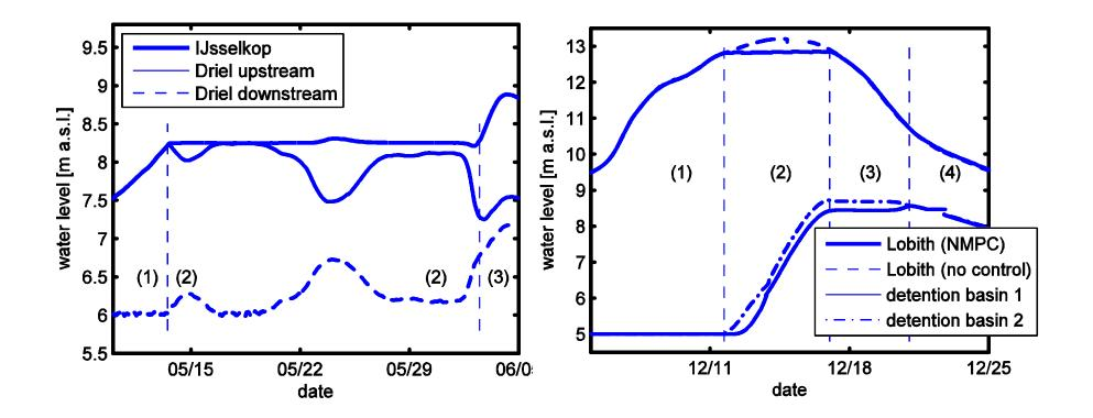
damping of small flood peak above 12.75 m a.s.l. in December 2007 at gauge Lobith by control of detention basins 1 and 2
