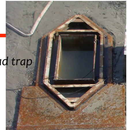
sill with geophone plates
